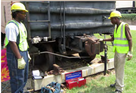
Students Nathaniel Jackson and Damaseni Ntahimpera demonstrate parts of "coupler" on a rail car.
