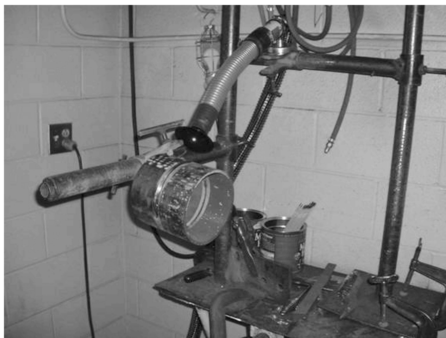
FIGURE 1. Pipe section and hood placement used in the experimental setting
