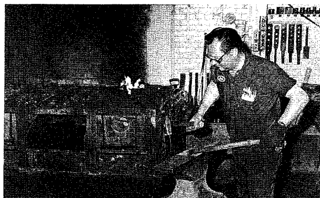
Blacksmithy —Dennis Kaminski is one of two blacksmiths employed by Consolidated Papers, Inc. They custom-make many brackets and parts for the complex paper-making machinery.
