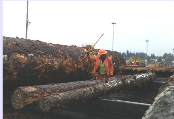
Bret Duvall, Local Lodge W130, is looking for rot in the knots of a spruce at Weyerhaeuser-Olympia, WA
